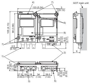
Dimensions of X when the video/RGB input unit is mounted to the GOT.
