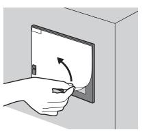
(2) Peel the release paper from the back of the new protective sheet, and attach its adhesive side to the GOT display
