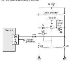
Power supply for loads connected to PLC output terminals
