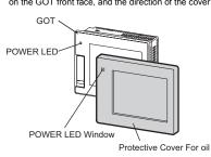
(2) One corner of the cover is pulled outside, and it hangs it on the corner of the front panel of GOT
