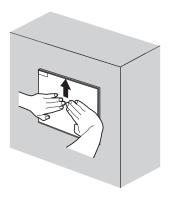
Remove the protective film from the protective sheet. When the user continues using the GOT with the protective film, the film may not be removed.
