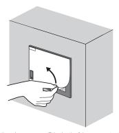
Peel the release paper off the back of the new protective sheet. With the protective film left on the sheet surface, attach the sheet on the GOT so that the USB environmental protection cover hole is just on the USB environmental protection cover of
