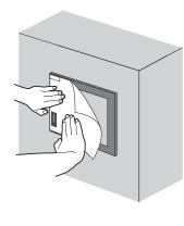
When attaching the protective sheet, make sure to fit the sheet on the GOT without leaving any clearance between the sheet and the GOT.
