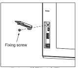
3) Tighten the screw with a torque of 0.36 N·m to 0.48N·r
