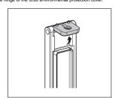
2) Put the provided fixing screw through the hinge hole. Fit the hinge projections of the USB environmental protection cover in the GOT guiding holes and fit the fixing screw of the USB environmental protection cover in the USB environmental protection cover installation hole on the GOT.
