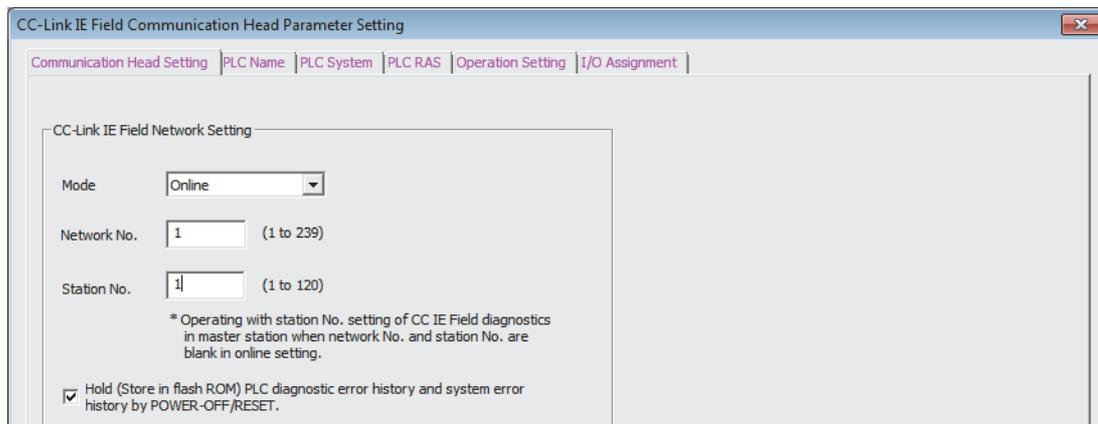
The "CC-Link IE Field Communication Head Parameter Setting" window. It has tabs for "Communication Head Setting", "PLC Name", "PLC System", "PLC RAS", "Operation Setting", and "I/O Assignment". The "Communication Head Setting" tab is active, showing the following settings:
