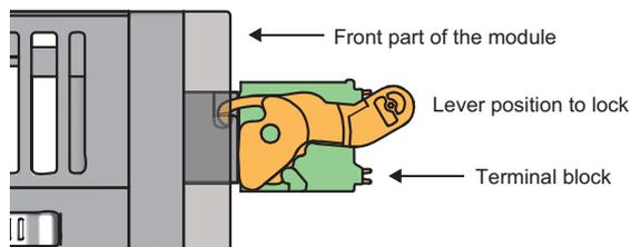
Figure from the top of the module: When the terminal block is installed
