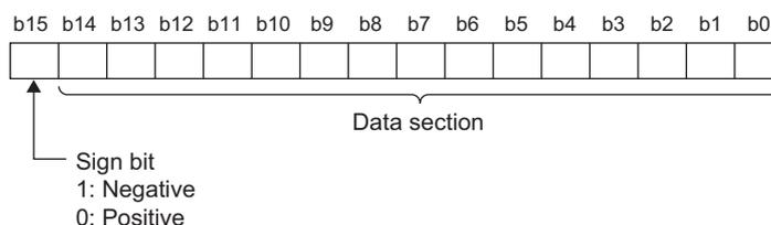
A value on which the set shifting amount to conversion value is reflected is stored in CH□ Digital operation value (Un\G54 to Un\G61).
