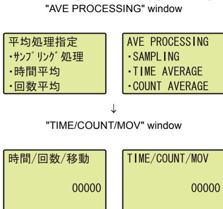
1. Select "SAMPLING", "TIME AVERAGE", "COUNT AVERAGE", or "MOVING AVERAGE" with the ▲ or ▼ button and confirm with the
