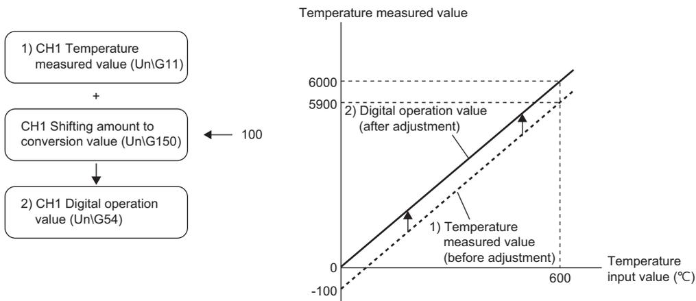
**Ex.** To set the shifting amount to conversion value to "5000" for the module to which Pt100 (-200 to 850°C) is set as the input range
