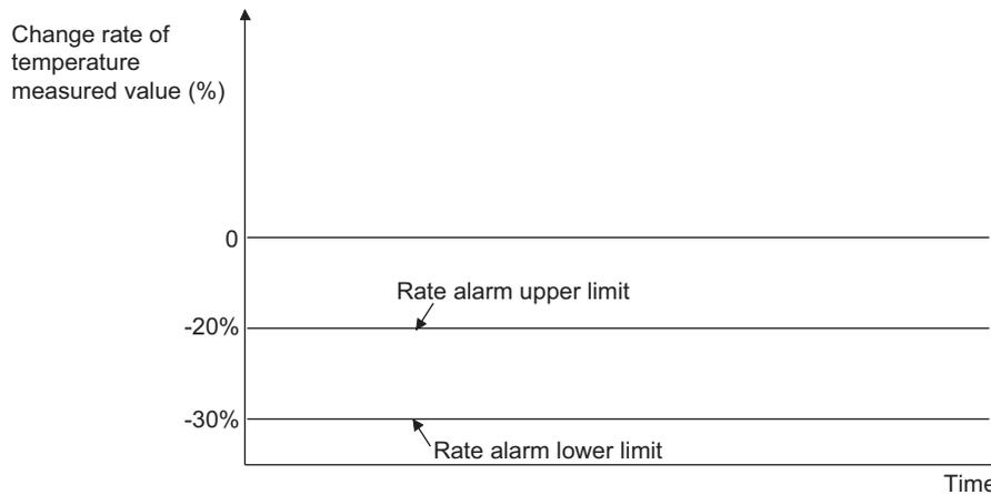
**Ex.** Monitoring whether the change rate of a temperature measured value lies within a specified range
