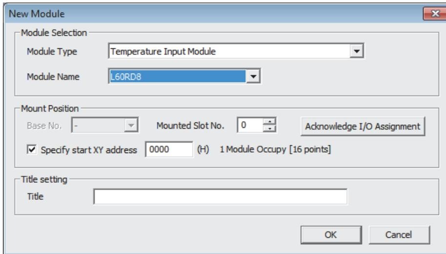
**4. Display the initial setting window for the RTD input module (L60RD8) and configure the setting as follows.**
