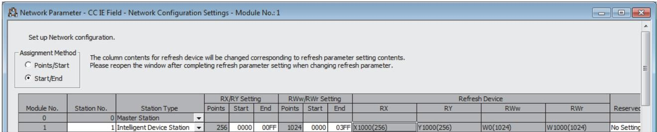
**4. Display the Refresh Parameters window and configure the setting as follows.**
