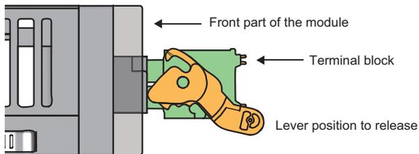
Figure from the top of the module: When removing the terminal block
