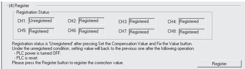
**22.** After the correction values have been determined, "Registration Status" of the target channels is shown as Unregistered.
