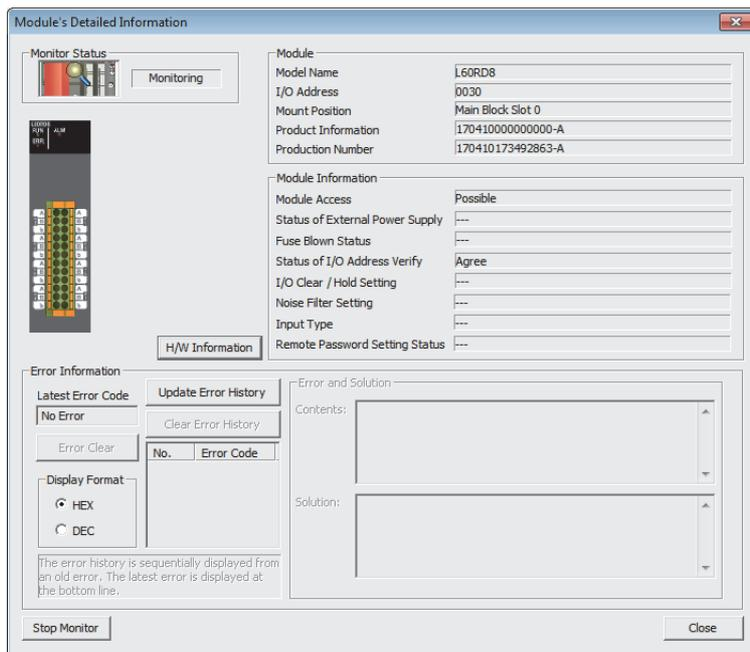
2. "Module's Detailed Information" of the RTD input module is displayed.
