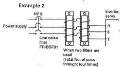
Wind the 3-phase wires all in the same direction with the same number of windings, and insert into the inverter and servo power input side.
