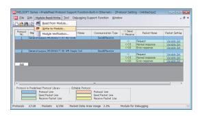
6. Write the protocol setting data to the CPU module.
