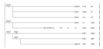
8. Create a program for starting data communications. In the case of Active open, create the program in which SP.SOCOPEN instruction is used to establish a connection. ( Page 77, Section 7.4.1)
