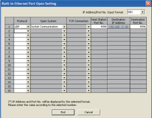
• For the "Ethernet Conf.", drag and drop the "General Socket UDP Module" from "Module List" to the left side on the window. Set port numbers and IP address as mentioned below.
