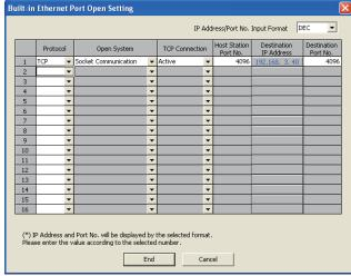
• For the "Ethernet Conf.", drag and drop the "General Socket Active Module" from "Module List" to the left side on the window. Set port numbers and IP address as mentioned below.
