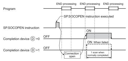
A connection with no parameters (no protocol is specified) can be opened. In this case, specify 8000<sub>H</sub> for \$\mathbb{G}\$ +0 and configure open settings in \$\mathbb{G}\$ +2 to \$\mathbb{G}\$ +9.
