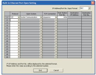
For the "Ethernet Conf.", drag and drop the "General Socket Fullpassive Module" or "General Socket
