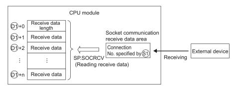
The result of the SP.SOCRCV instruction can be checked with the completion device 2+0 and 2+1.
