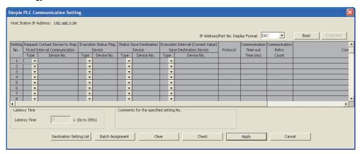
Simple PLC Communication Setting consists of Base Setting (essential) and Extended Setting (optional). To switch the window, use the Basic / Extended button on the top right of the window.
