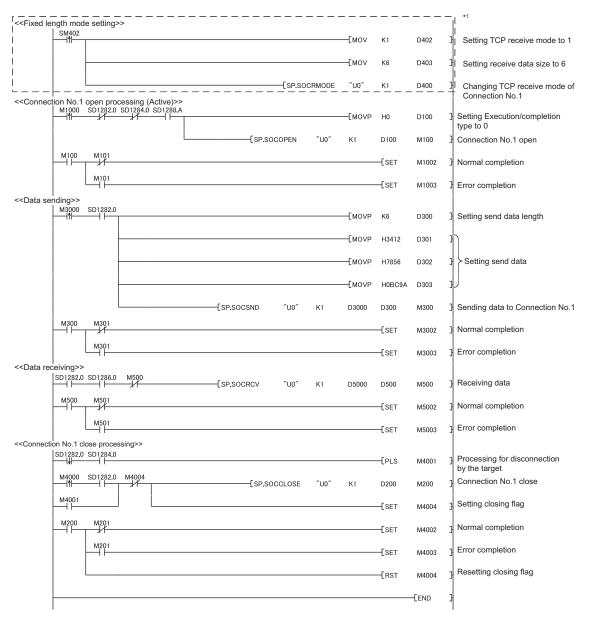
\*1 There are two kinds of TCP receive modes: TCP standard receive mode and TCP fixed-length receive mode. For fixing the data size, run the program enclosed by a dotted line.
