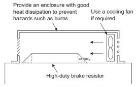
How to Install the Resistor
