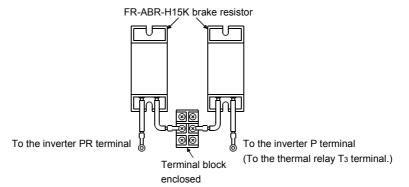
• If you extend the high-duty resistor lead wire to use, use the wire with a size as noted below and not exceeding 5m in length. Installation shall be in accordance with the North American or Canadian Electrical Code and any applicable provincial codes (codes of each state).
