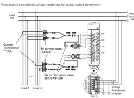
\*For a low voltage circuit, grounding of the secondary sides of VT is not necessary.
