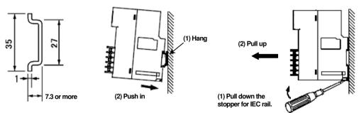
To install IEC rails, secure them using M4 or M5 screws at intervals of 25 to 100 mm. When installing IEC rails in series, secure each end of the IEC rails with sideslip prevention clamps. When reinstalling the product onto an IEC rail after removal, install it with the IEC rail stopper pushed in upward.
