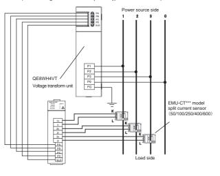
Input signal wire shall not be bound together with or placed close to the main circuit and power
