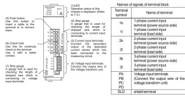
Check the stripping length using the strip gauge of QE81WH4W main module
