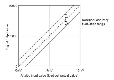
When the rated output of a load cell is 2mV/V, the zero drift, gain drift, and integrated accuracy are calculated by the following equations:
