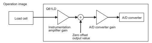
While a load cell of which rated output is 3.0mV/V or less may be connected to the Q61LD, the input range available for conversion (with no conversion over error) depends on the combination of Instrumentation amplifier gain setting (Un\G80) and A/D converter gain setting (Un\G81).
