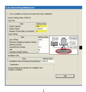
Set "Rated Capacity" to 250, "Rated Output" to 2.0mV/V, and "Number of load cells in connection" to 4.
