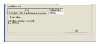
3. Set the value for "Installation Site Gravitational Acceleration" and click the setting range of gravitational acceleration is 9.7000 to 9.9999.
