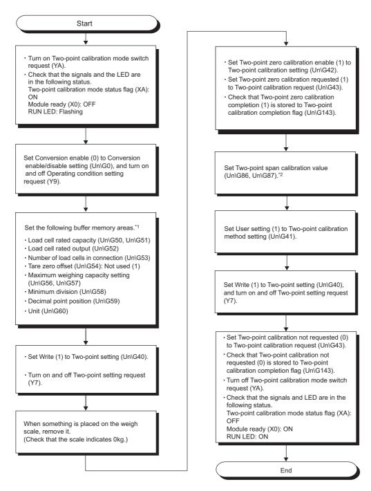
Configure the setting the same as when executing actual load calibration.
