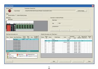
1. Open the "System Monitor" window of the remote I/O station.
