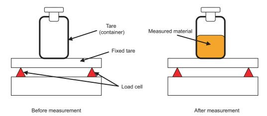
The net weight (NET) can be calculated from Gross weight output value (Un\G100, Un\G101) by using the following method:
