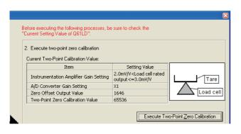
With nothing placed on the weighing machine (0kg) except for the fixed tare, click the
