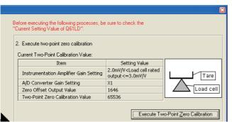
3. With nothing placed on the weighing machine (0kg) except for the fixed tare, click the
