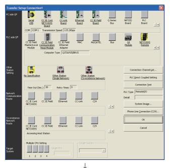
4. Set it to enable access to the modules of the remote
