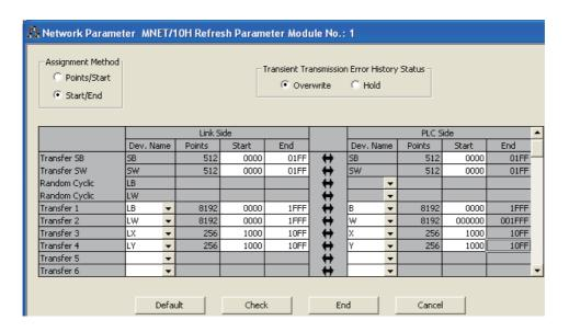
**5.** Write the set parameters to the CPU module of the master station. Then reset the CPU module or power off and on the programmable controller.
