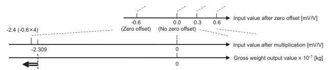
When the load on the load cell is completely eliminated by removing the fixed tare, the zero offset output value (-0.6mV/V) is multiplied by 4 in A/D converter gain. Although, the converter input value exceeds the conversion range on the minus side.
