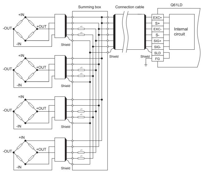
\*1 The averaging resistors (R) must have the resistance value of 300 to  $500\Omega$  with an excellent temperature coefficient (e.g., the ppm/°C value must not be better than that of the module performance), and the relative ratio must be equal among the resistors.
