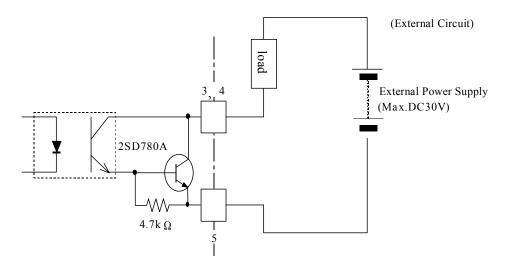
Figure 5.3 Output Circuit
