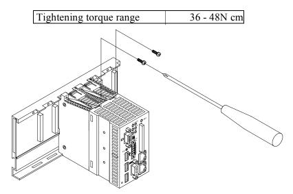
Figure 3.2 Installing the Module 2
