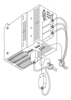
Figure 3.5 The hole to attach the binding tie
