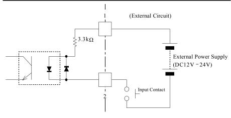
Figure 5.2 Input Circuit
