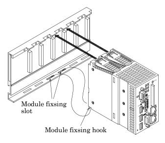
Figure 3.1 Installing the Module 1
