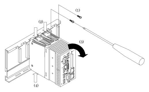
Figure 3.3 Uninstalling the Module
