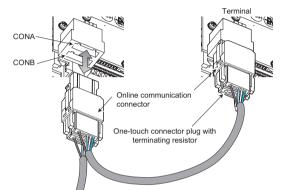
Use the following online communication connector and one-touch connector plug with terminating resistor.
