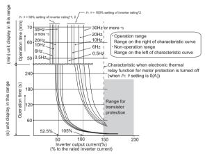
This function detects the overload (overheat) of the motor, stops the operation of the inverter's output transistor, and stops the output.
