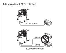
When driving a 400V class motor by the inverter, surge voltages attributable to the wiring constants may occur at the motor terminals, deteriorating the insulation of the motor. Take the following measures (1) or (2) in this case.
