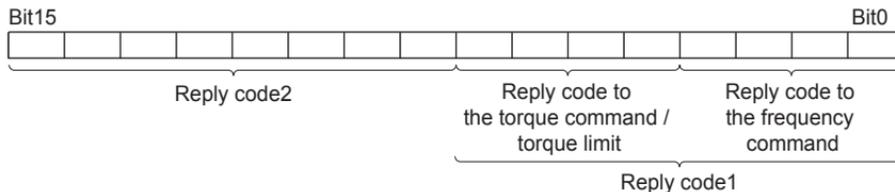
Example) The error code is H0030 when the torque command value is outside the setting range.
