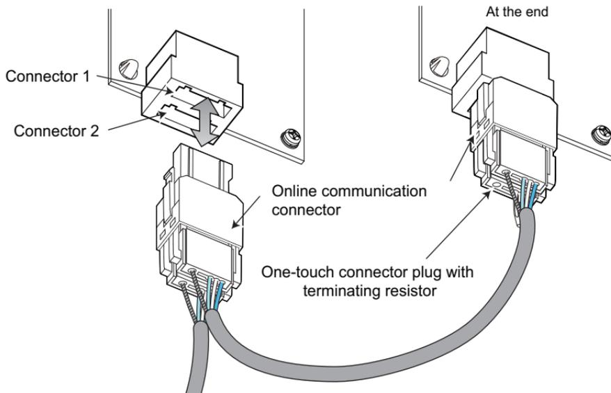
Use the following online communication connector and one-touch connector plug with terminating resistor.
