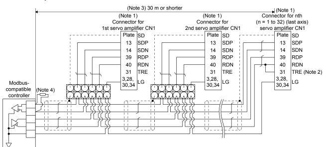
Note 1. Connector set MR-J3CN1 (3M or equivalent) Connector: 10150-3000PE
