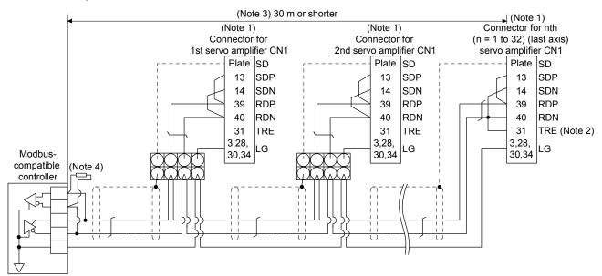
Note 1. Connector set MR-J3CN1 (3M or equivalent) Connector: 10150-3000PE Shell kit: 10350-52F0-008
