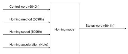
Note. In the point table mode, use the acceleration time constant and deceleration time constant in point table No. 1 (2801h).
