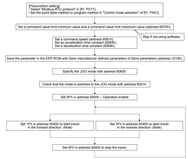
Note. [The operations are performed when [Pr. PT01] (address 2481h) is set to "\_\_\_1" (incremental value command method). When [Pr. PT01] (address 2481h) is set to "\_\_\_0" (absolute value command method), setting 1Fh in address 6040h starts travel to the target position.
