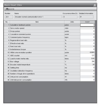
(c) Click the History Clear button to delete all data at alarm occurrence recorded in the servo amplifier. After clicking the History Clear button, cycle the power of the servo amplifier. This restart takes longer time than usual due to the deletion of data.
