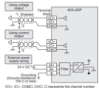
\*1 Use 2-core shielded twisted pair cable for the analog output lines, and separate the analog output lines from other power lines or inductive lines.
