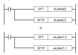
To shift the bits correctly, specify the array of a bit type label.
