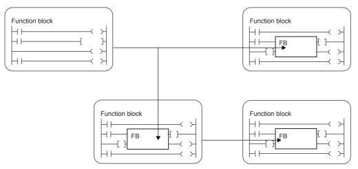
Unlike the function, the function block does not output return values.
