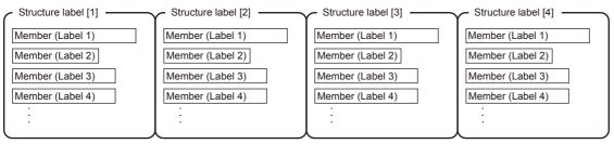
When a structure is declared as an array, append an index enclosed by "[]" after the structure label name. The array of structure can be specified as arguments of functions and function blocks.
