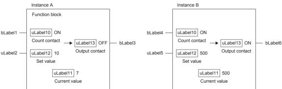
The above function block starts counting current value when the input variables (Count contact) turn on and turns on the output variable (Output contact) when the current value held in the internal variable reaches the set value.
