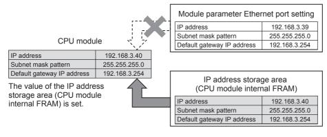
[In the case Module parameter Ethernet port setting is used (IP address storage area is cleared)]
