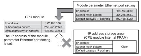
When IP address storage area is cleared (IP address change function enable flag SM8498 is OFF), module parameter Ethernet port setting is enabled.
