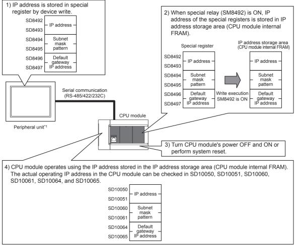
\*1 The IP address change function can be used not only by peripheral units but also by link function, MX Component and MX Sheet by manipulating values of the special devices. For details on link function, refer to the IIMELSEC iQ-F FX5 User's Manual (Serial Communication). For details on MX Component and MX Sheet, refer to the IIMespective product manual.
