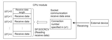
The result of the SP.SOCRCV instruction can be checked with the completion device (d2)+0 and (d2)+1.
