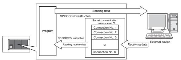
\*1 The area is used for storing data received from the connected open devices.
