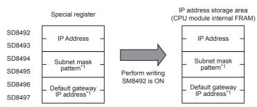
\*1 It is possible to specify no setting (0.0.0.0) for the subnet mask pattern and default gateway IP address. However, it is necessary to specify no setting (0.0.0.0) for both the subnet mask pattern and the default gateway IP address. If no setting (0.0.0.0) is specified for only one, an error will occur and the IP address will not be changed.
