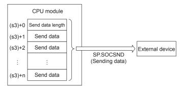
The result of the SP.SOCSND instruction can be checked with the completion device, (d)+0 and (d)+1.
