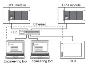
The flow up to start of Ethernet communication by the connection via a hub is as follows.
