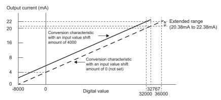
The current 22.00mA corresponding to the digital value 36000, which is the sum of 'CH1 Digital value' (Un\G460) and the input value shift amount, is output and the analog values corresponding to the extended part of the extended mode can be output.
