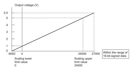
The digital value 27000 corresponds to the analog output voltage 5.5V. Thus, the analog values corresponding to the extended range can be output by setting 'CH1 Digital value' (Un\G460).
