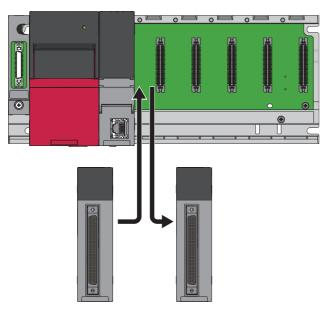
**2.** Power off the programmable controller and replace the D/A converter module with a new one.
