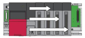
**5.** Apply the offset/gain values to modules No.2 to No.4
