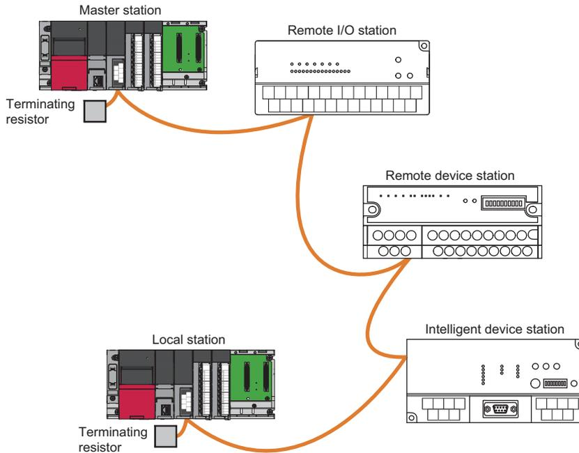
The CC-Link version and the number of slave stations that can be connected vary depending on the mode of the master/local module. (☞ Page 19 Maximum Number of Connectable Modules)
