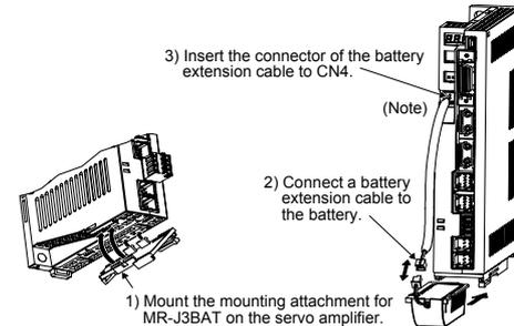
Note. Be careful not to catch battery extension cable on peripheral equipment or by your fingers. Doing so may cause a disconnection of the CN4 connector due to stress on the connector connection part.
