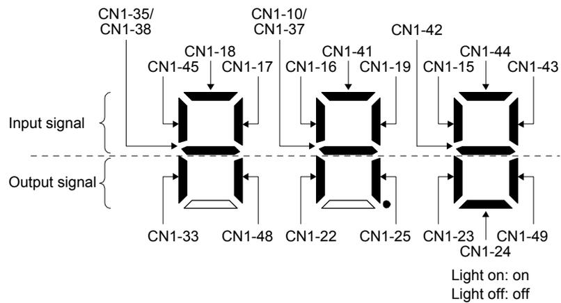
The LED segment corresponding to the pin is lit to indicate on, and is extinguished to indicate off. The decimal point in the second digit flickers continuously.
