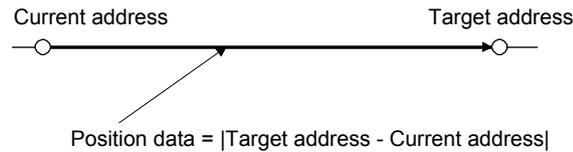
This section indicates contents different from the absolute value command method (factory setting) when this servo amplifier is used under the incremental value command method.
