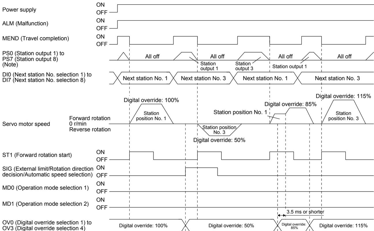
Note. For MR-J4-03A6-RJ servo amplifiers, up to six points of DO are available; therefore, PS0 to PS7 cannot be outputted simultaneously.
