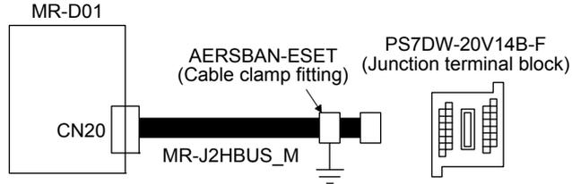
Ground the option cable on the junction terminal block side with AERSBAN-ESET (cable clamp fitting). For how to use the cable clamp fitting, refer to section 11.14 (2) (c) of "MR-J4-\_A\_(-RJ) Servo Amplifier Instruction Manual".
