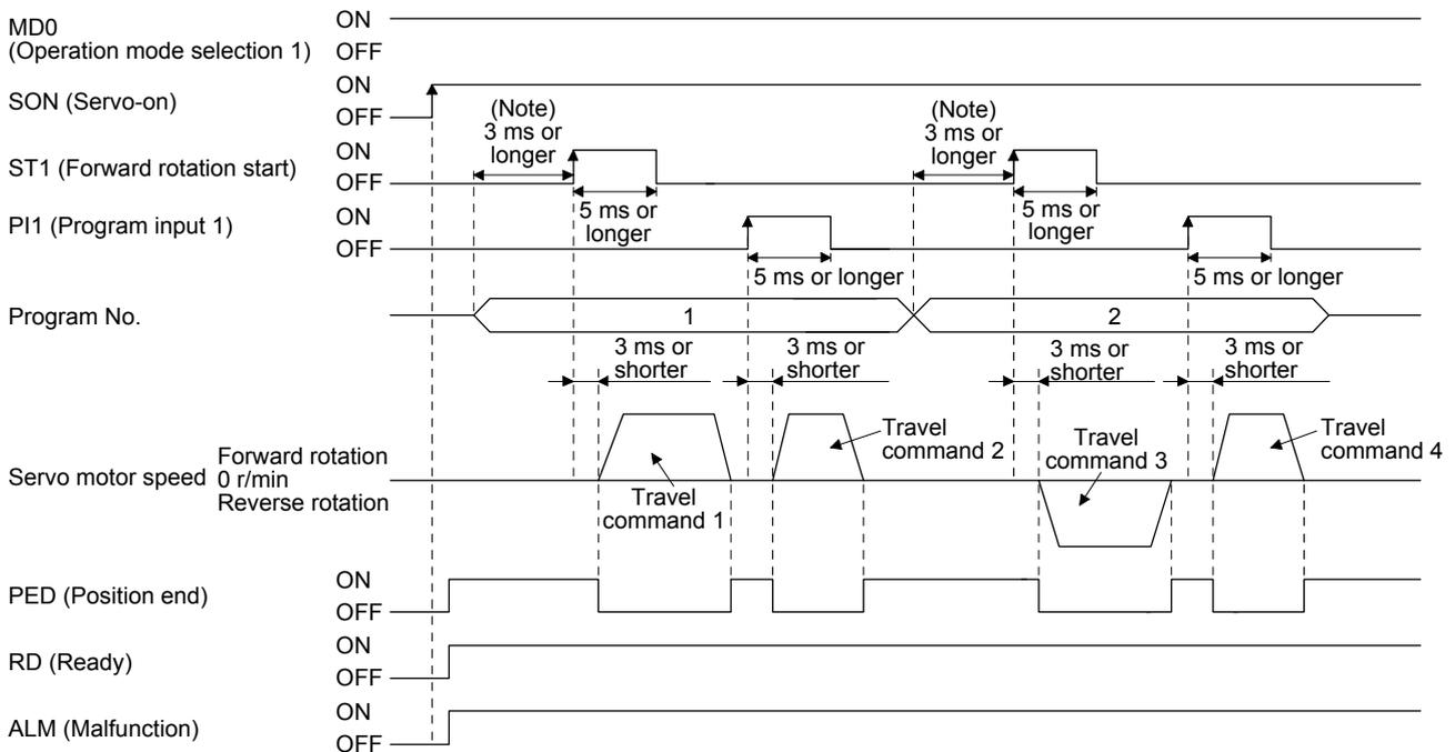
Note. The detection of external input signals is delayed by the set time in the input filter setting of [Pr. PD29]. Considering the output signal sequence from the controller and signal variations due to hardware, configure a sequence that changes the program selection earlier.
