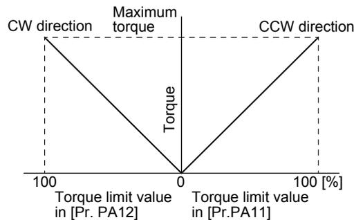
A relation between the applied voltage of OTLA (Analog torque limit) and the torque limit value of the servo motor is as follows. Torque limit values will vary about 5% relative to the voltage depending on products. At the voltage of less than 0.05 V, torque may vary as it may not be limited sufficiently. Therefore, use this function at the voltage of 0.05 V or more.
