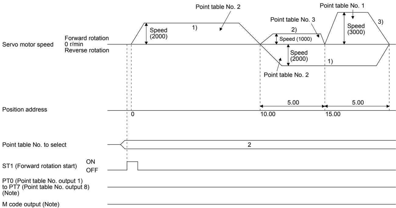
Note. PT0 to PT7 and M code are not outputted in automatic continuous operation.
