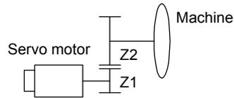
Pt (Servo motor resolution): 4194304 pulses/rev
