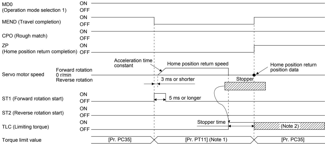
Note 1. The following torque limits are enabled.
