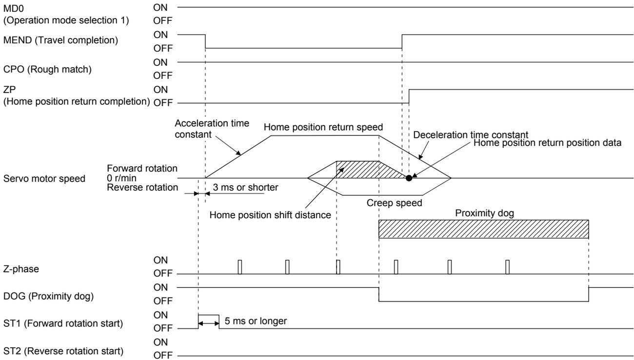
The setting value of [Pr. PT08 Home position return position data] is used as the position address at the home position return completion.
