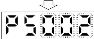
When the lower three digits flicker, press the "SET" button to complete the teaching setting preparation. The upper two digits on the display will flicker on completion of proper preparation
