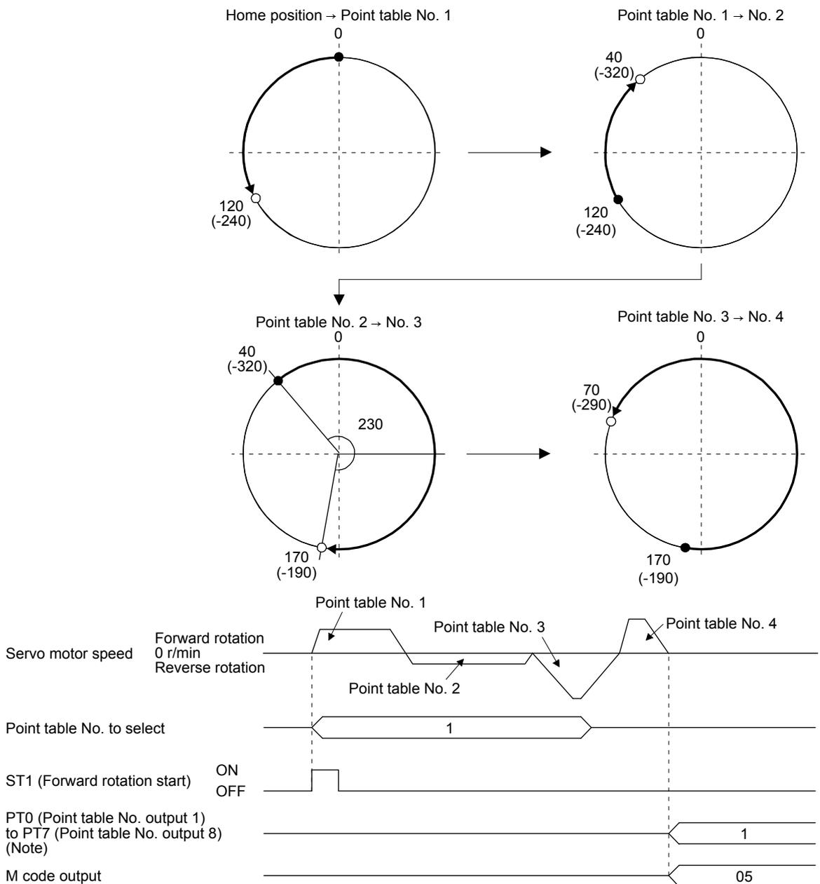
Note. For MR-J4-03A6-RJ servo amplifiers, up to six points of DO are available; therefore, PT0 to PT7 cannot be outputted simultaneously.
