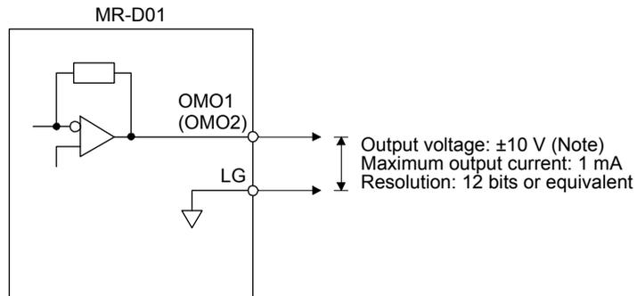
Note. Output voltage range varies depending on the monitored signal. When connecting analog output to an external device, use the withstand voltage of 15 V DC or higher.
