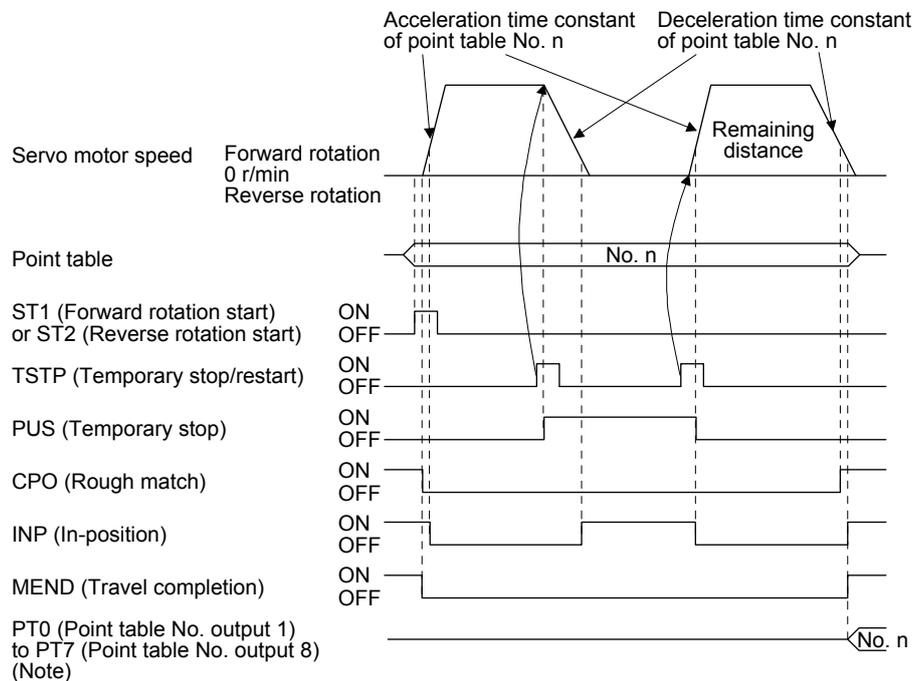
Note. For MR-J4-03A6-RJ servo amplifiers, up to six points of DO are available; therefore, PT0 to PT7 cannot be outputted simultaneously.
