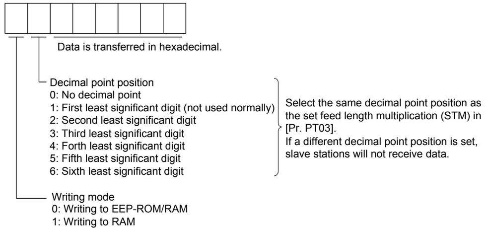
When the position data is changed frequently using communication, set "1" to the mode to change only the RAM data in the servo amplifier.
