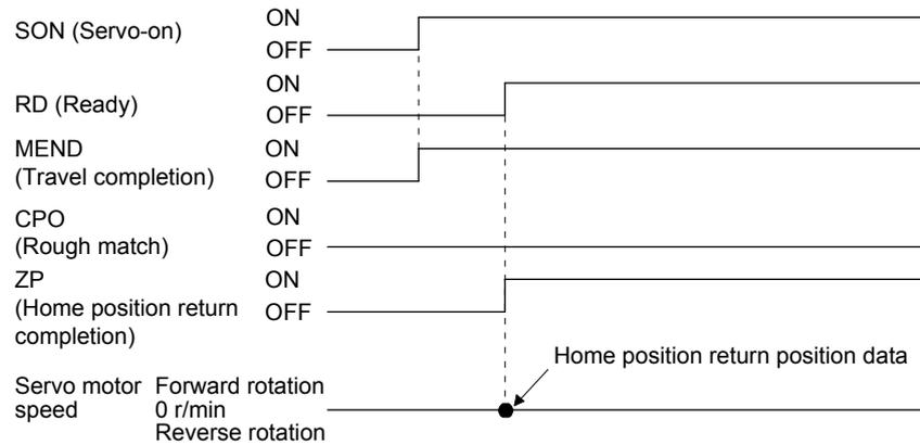
The setting value of [Pr. PT08 Home position return position data] is used as the position address at the home position return completion.
