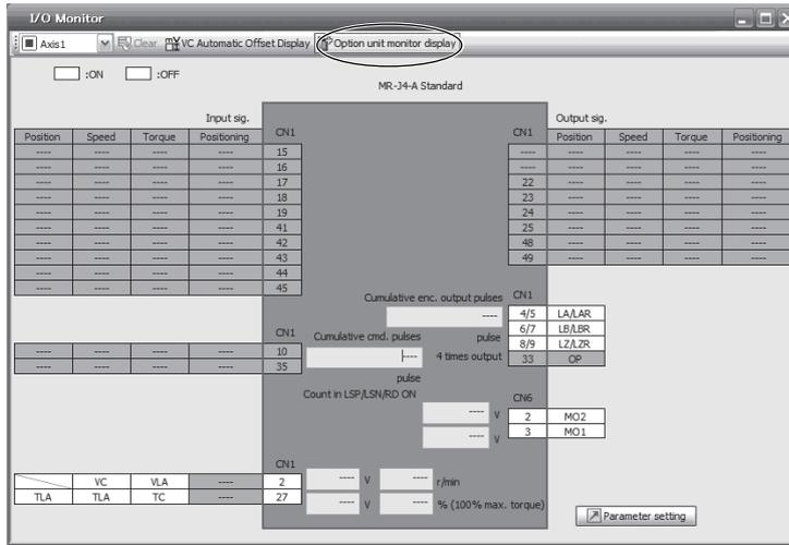
The following window is displayed. The input/output monitor on the MR-D01 side can be checked.
