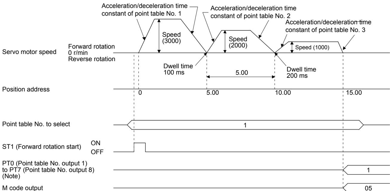
Note. For MR-J4-03A6-RJ servo amplifiers, up to six points of DO are available; therefore, PT0 to PT7 cannot be outputted simultaneously.
