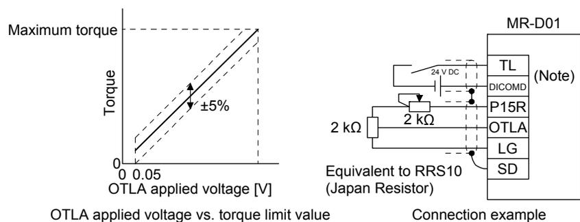
Note. This diagram shows sink I/O interface. For source I/O interface, refer to section 11.5.5 (5).
