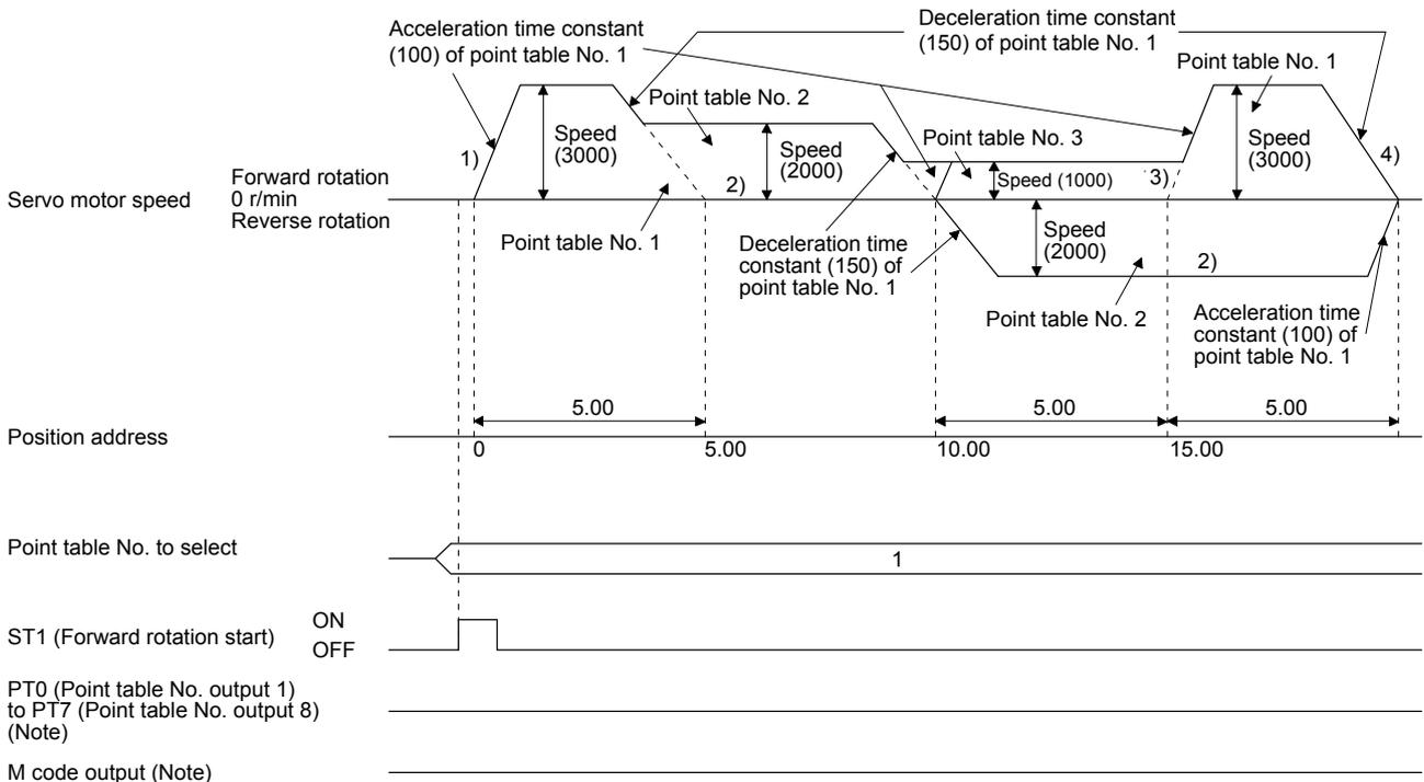
Note. PT0 to PT7 and M code are not outputted in automatic continuous operation.
