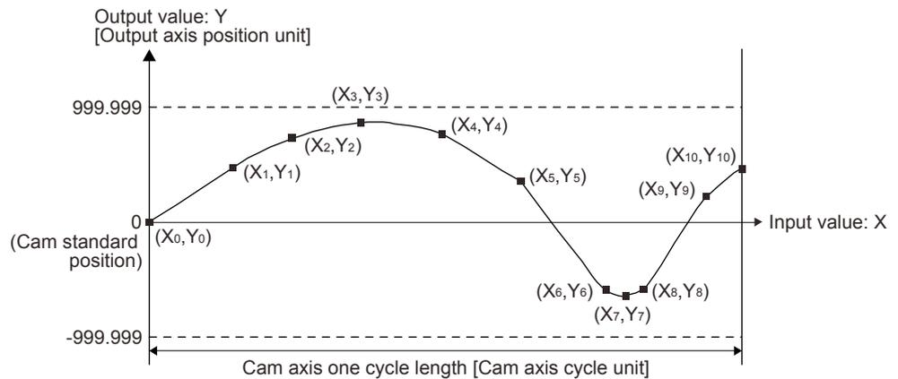
If "input value = 0" and "input value = cam axis one cycle length" are not set in the coordinate data, a control is executed by the line connecting the closest two points.
