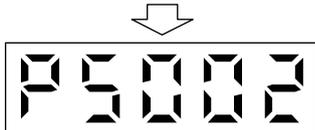
When the upper two digits or the lower two digits flicker, the display returns to the teaching setting initial screen by pressing the "MODE" button.
