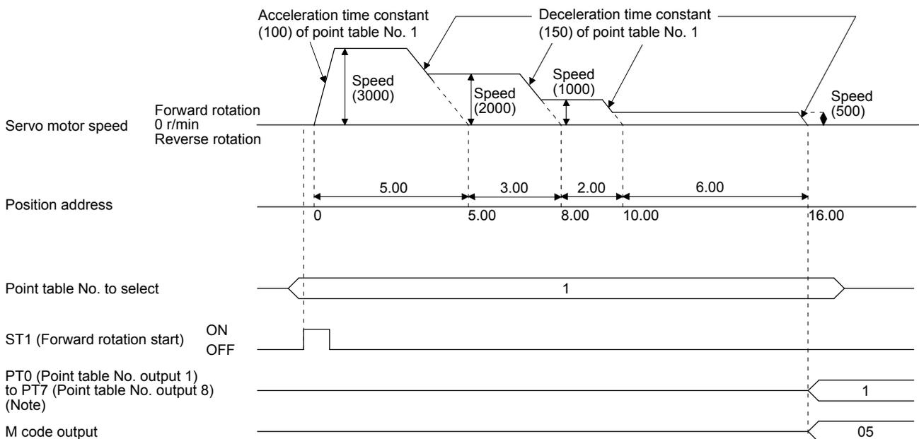
Note. For MR-J4-03A6-RJ servo amplifiers, up to six points of DO are available; therefore, PT0 to PT7 cannot be outputted simultaneously.
