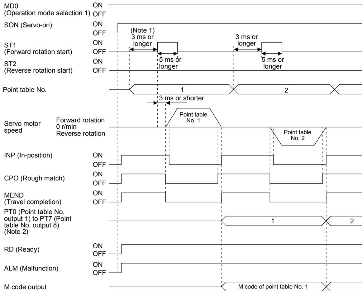
Note 1. The detection of external input signals is delayed by the set time in the input filter setting of [Pr. PD29].
