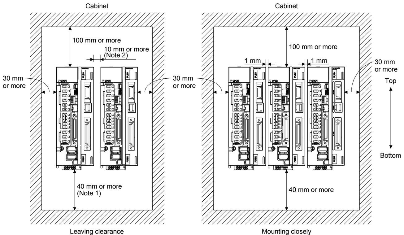
Note 1. For the 11 kW to 22 kW servo amplifiers, the clearance between the bottom and the ground will be 120 mm or more.
