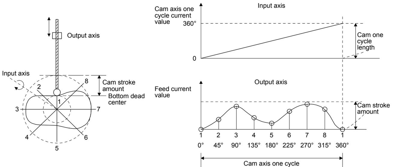
By setting cam data and cam control data, the simple cam function enables synchronous control with an input axis (external pulse command input, point table command, or program positioning command) with a start of positioning.
