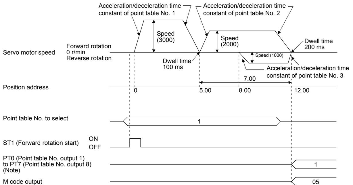
Note. For MR-J4-03A6-RJ servo amplifiers, up to six points of DO are available; therefore, PT0 to PT7 cannot be outputted simultaneously.
