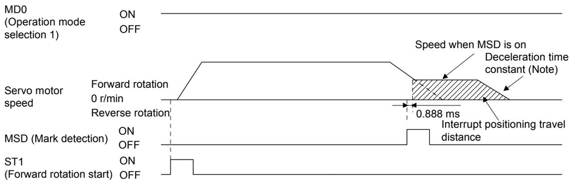
Note. Deceleration time constant of the point table at the time of start is applied for the point table method, and deceleration time constant set by the program in execution is applied for the program method.
