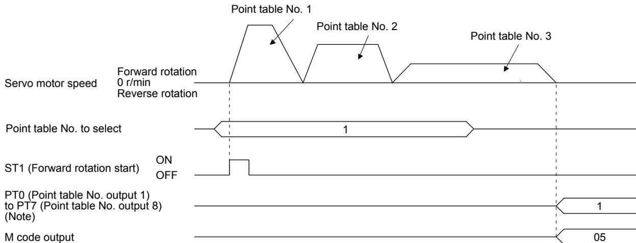
Note. For MR-J4-03A6-RJ servo amplifiers, up to six points of DO are available; therefore, PT0 to PT7 cannot be outputted simultaneously.
