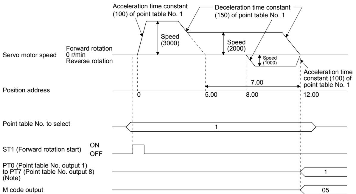
Note. For MR-J4-03A6-RJ servo amplifiers, up to six points of DO are available; therefore, PT0 to PT7 cannot be outputted simultaneously.
