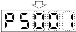
When the lower three digits flicker, press the "UP" or "DOWN" button to select the point table.
