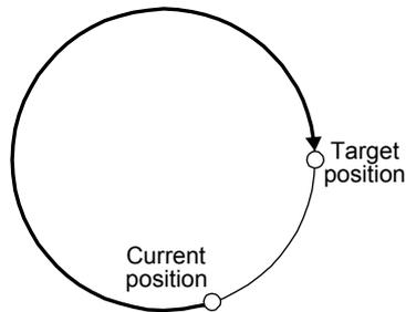
When the position data of -360.000 degrees is specified, the servo motor rotates in the CW direction. (A)
