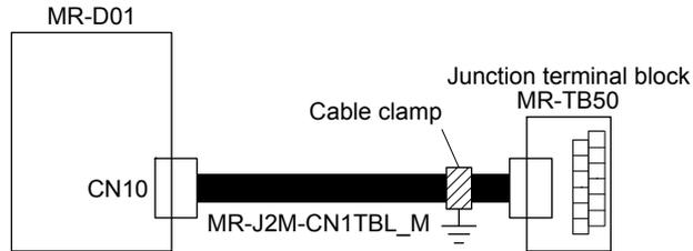
Ground the junction terminal block cable on the junction terminal block side with the supplied AERSBAN-ESET (cable clamp fitting). For how to use the cable clamp fitting, refer to section 11.14 (2) (c) of "MR-J4-\_A\_(-RJ) Servo Amplifier Instruction Manual".
