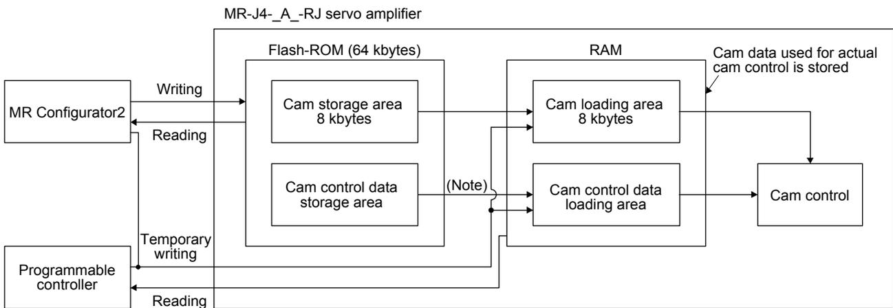
Note. When the power is turned on, the cam data and the cam control data are copied from the Flash-ROM to the RAM.
