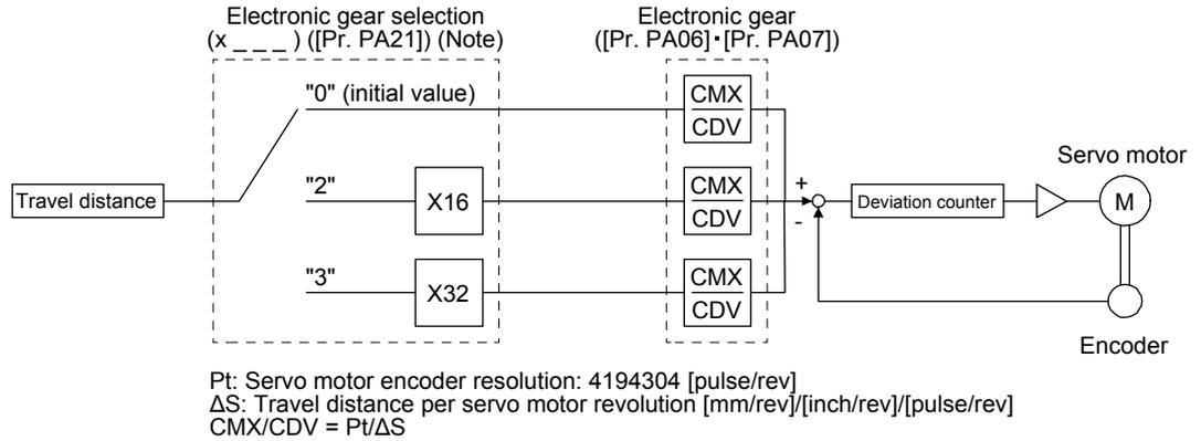
Note. For MR-J4-03A6-RJ servo amplifiers, "2 \_\_\_" or "3 \_\_\_" cannot be set to [Pr. PA21].
