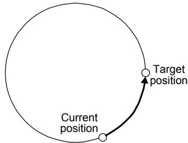
When the position data of -90.000 degrees is specified, the servo motor rotates in the CW direction.
