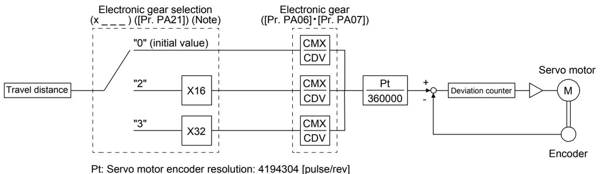
Note. For MR-J4-03A6-RJ servo amplifiers, "2 \_\_\_" or "3 \_\_\_" cannot be set to [Pr. PA21].
