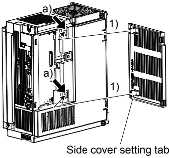
1) Insert the side cover setting tabs into the sockets a) of the servo amplifier.
