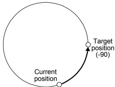
If the position data of 270.000 degrees is specified when the current position is at 90, the distances in the CCW and CW are the same. In such a case, the servo motor rotates in the CCW direction.
