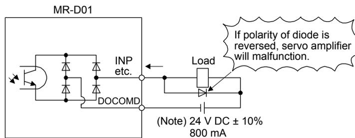
Note. If the voltage drop (maximum of 2.6 V) interferes with the relay operation, apply a high voltage (maximum of 26.4 V) from an external source.
