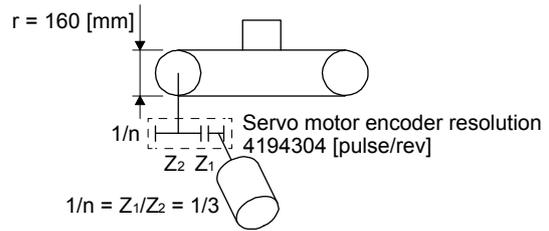
Servo motor encoder resolution  $P_t = 4194304$  [pulse/rev]
