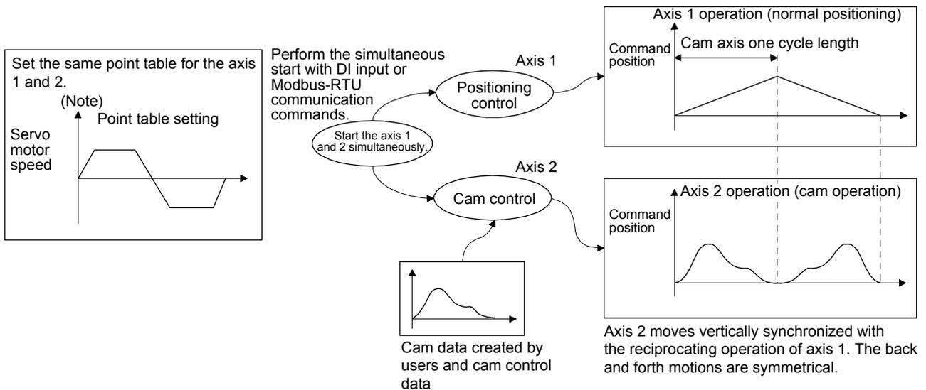
Note. Input the same positioning commands (point table data) to the driven shaft (axis 2) as those for the main shaft (axis 1).
