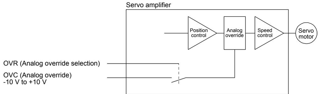
Select a changed value by using OVR (Analog override selection).
