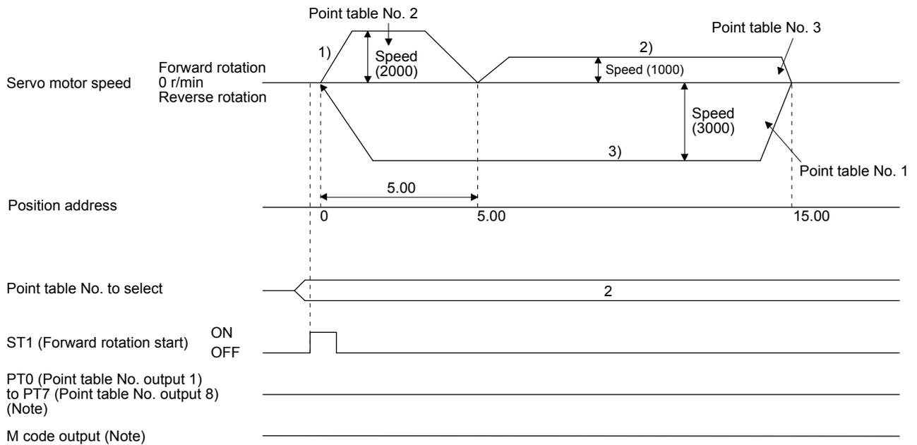
Note. PT0 to PT7 and M code are not outputted in automatic continuous operation.
