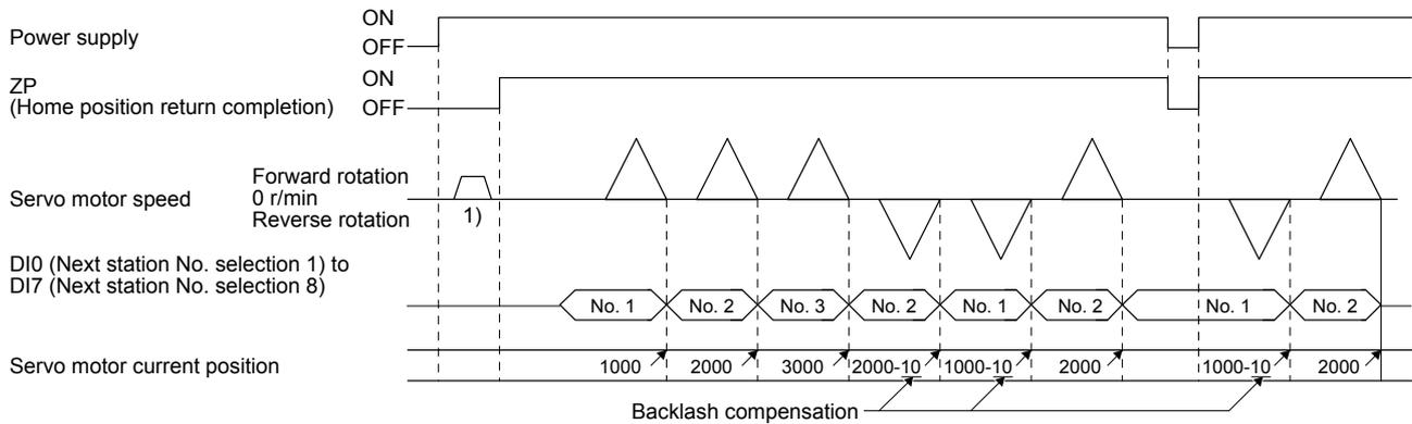
Backlash is compensated to the direction set with [Pr. PT38] regardless of a JOG operation ( 1)) or disturbance after power-on.
