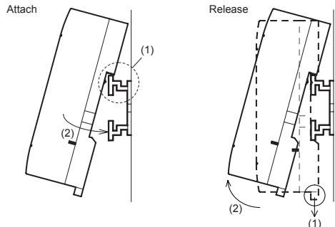
**ENG** When installing the AL2-2PT-ADP module refer to Figure 2.
