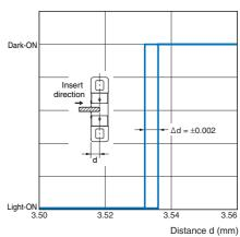
Vcc = 24 V, No. of repetitions: 20, Ta = 25°C Differential distance = 0.025 mm max.
