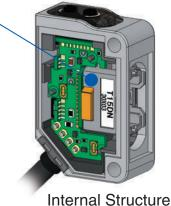
miniaturization is obvious in the photo IC, which includes an external light interference prevention algorithm, CSP\* mounting, and other components.
