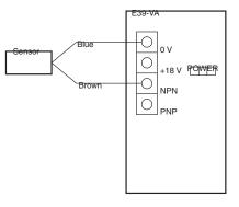
18 V (use two 9-V dry-cell batteries) Operates when the output transistor of
