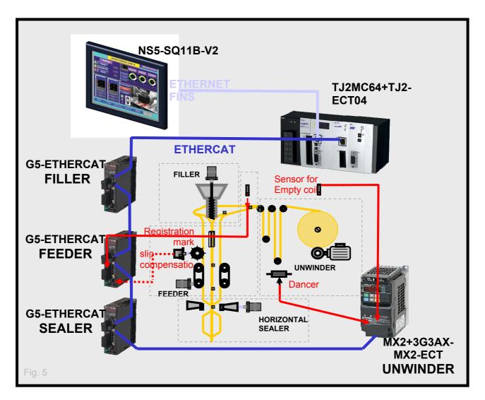
The proposed solution is based on the TJ2-MC64 motion controller with the TJ2-ECT04 EtherCAT Master. The filler, feeder and sealer will be driven by G5 servodrives with EtherCAT interface and the unwinder will be a MX2 Inverter, also with EtherCAT option board.
