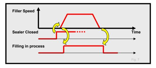
**Note**: in this entire document we will draw the speed time curve because it is easier to visualize but the commands we give are POSITION. The position in this graph is the area below the speed curve.
