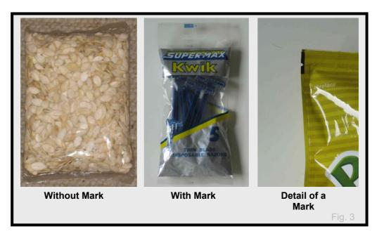
Most of the machines have the option to work with mark and without mark.
