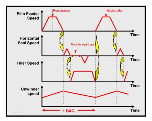
The next diagram shows the sequence of a complete cycle:
