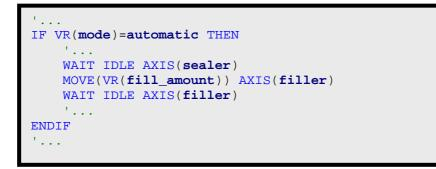
The variables grouped as VR(name) are global variables that may be changed via the HMI. Those variables can be changed and applied on the fly, depending on the way the program is written.
