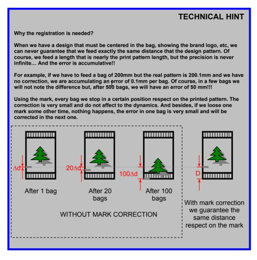
If the mark is in such a position that is detected just at the end of the bag, it may happen that sometimes is detected at the end of the current bag and sometimes at the beginning of the next one. It is better to avoid this situation, otherwise, it needs additional program code to distinguish between both situations and make the right processing:
