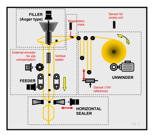
Some parts of the machine are a must; some other varies depending on the material used in the bags and on the goods to be packed.
