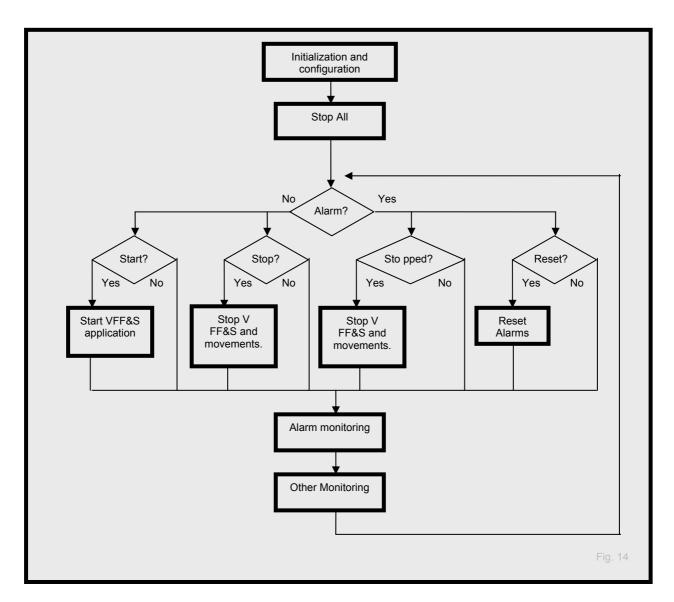
As you can see from section 3, making an application program for the Vertical Form Fill and Seal is not complicated. Sometimes it is more time consuming to program all the sequence around the cyclic machine operation, that is:
