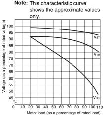
Motor load (as a percentage of rated load) Note: For phase loss of phase R. V<sup>ST</sup>, V<sup>TR</sup>, and V<sup>RS</sup> indicate the motor terminal voltage at phase loss.
