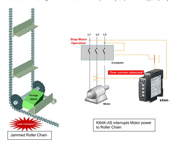
By using the K8AK-AS3 the system automatically detects this increase in current caused by the jam and shuts down the roller chain operation. Once the jam is removed or cleared the system can be restarted without any reset time.
