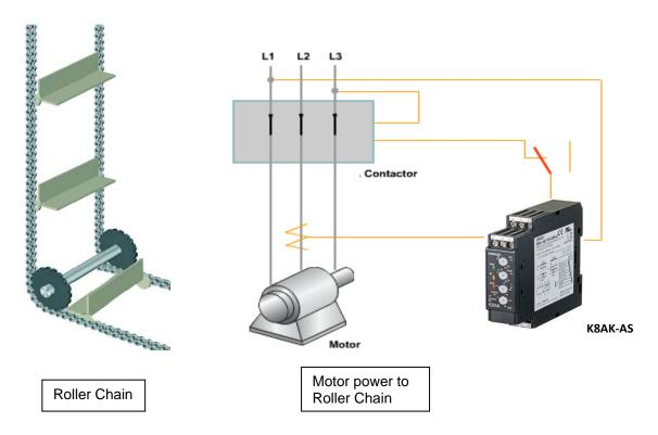
If a foreign object or the product on the conveyor jams the operation, the roller chain stops moving and the current level operating the motor will increase dramatically (Locked Rotor Condition). This locked rotor condition will damage the motor or break the chain (Conveory belt) if it is not stopped quickly.
