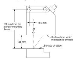
**Note:** Do not tighten the mounting screws for the moment as the optical axis must be adjusted.
