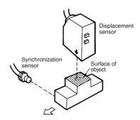
After the optical axis has been adjusted, tighten the mounting screws and secure the Synchronization Sensor firmly. Some Synchronization Sensor models incorporate a sensitivity controller. For the adjustment of such models, refer to the instruction manual for the Synchronization Sensor.
