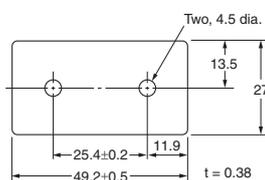
Note: 1. Each dimension has a tolerance of ±0.4 mm unless otherwise specified.
