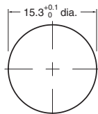
Panel Cutout Dimension Panel thickness = 1 to 4 mm
