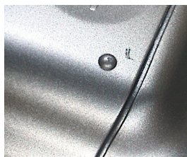
Defects in Molded Goods (Dents)
