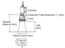
Note: The lengths of the fields of vision given in the optical charts are the lengths of the Y axis.
