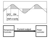
Enables precise temperature control and increases the heater's service life.
