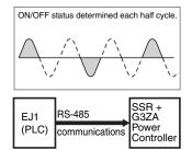
Many heaters can be control using communications. Enables noiseless operation with high-speed response.
