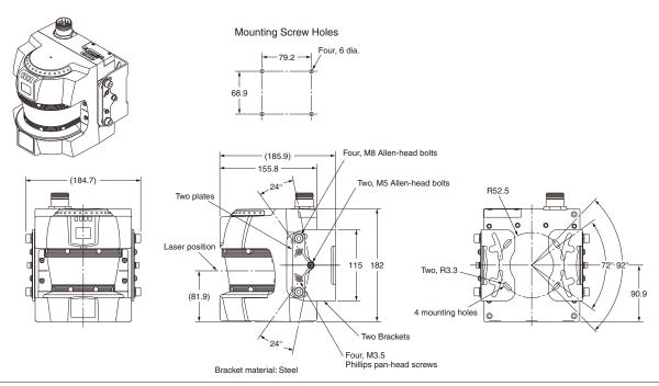
Safety Laser Scanner with L-shaped Mounting Brackets and Rear Surface Mounting Bracket 0S3101-2-PN-S + 0S3101-BKT + 0S3101-BPT
