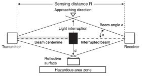
Fig. 2 Example of Unsafe Installation
