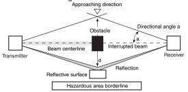
Fig. 3 Example of Unsafe Installation
