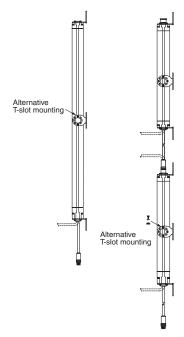
Note: When the alternate T-slot mounting is used to secure the MS/ MSF4800, the mounting bracket can no longer be used to adjust the beams.
