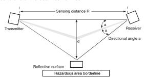
Fig. 5 Sensing Distance vs. Minimum Distance from the Reflective Surface
