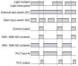
\* The output operation mode of the auxiliary output is the Dark-ON output mode
