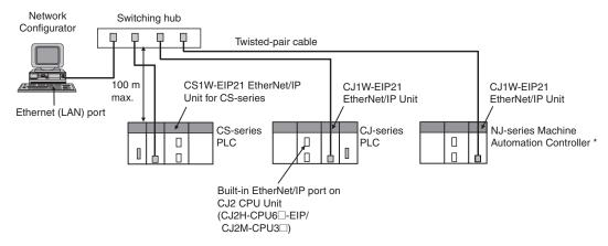
\* EtherNet/IP Unit with unit version 2.1 or later is required to connect C1JW-EIP21 to NJ-series CPU Unit. Use CPU Unit with version 1.01 or later and Sysmac Studio with version 1.02 or later.
