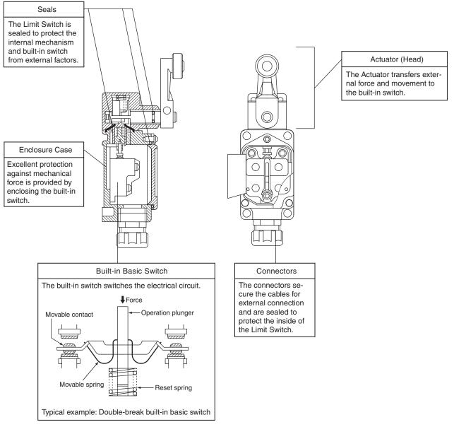
Structural Diagram of Typical Vertical Limit Switch
