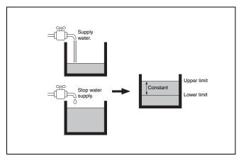
for electricity to flow) and the electrical current that flows in this circuit is used to detect the level of the liquid. A variety of conductive liquids can be controlled using this method. Detecting the resistance between the electrodes and comparing it to see if it is larger or smaller than a reference resistance is used to detect the surface of the liquid.
