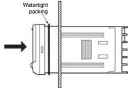
Insert the adapter into the grooves on the left and right sides of the rear case and push until it reaches the panel and is fixed in place.
