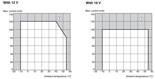
Note: 1. The above values are for standard mounting. The derating curve differs depending on the mounting conditions.
