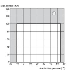
Note: 1. The above values are for standard mounting. The derating curve differs depending on the mounting conditions.
