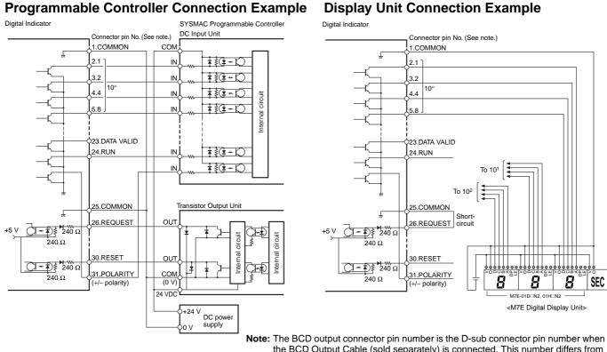
the BCD output connector pin number is the D-sub connector pin number when the BCD Output Cable (sold separately) is connected. This number differs from the pin number for the Digital Indicator narrow pitch connector (manufactured by Honda Tsushin Kogyo Co., Ltd.).
