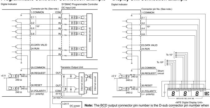
the BCD Output Cable (sold separately) is connected. This number differs from the pin number for the Digital Indicator narrow pitch connector (manufactured by Honda Tsushin Kogyo Co., Ltd.).
