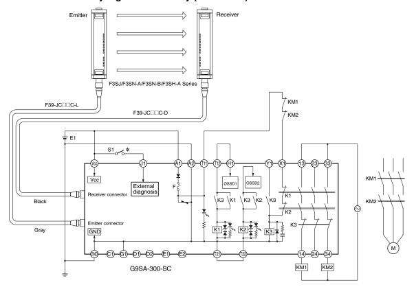
External test switch KM1 and KM2: Magnetic Contactors M: 3-phase motor
