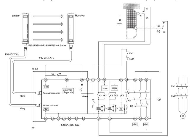
S1: Limit switch (NO) Safety Limit Switch with S2:
