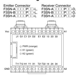
The pin arrangement at the Sensor is shown below.
