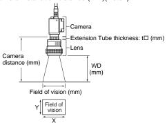
Note: 1. The lengths of the fields of vision given in the optical charts are the lengths of the Y axis.
