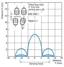
Note: Shading indicates the range in which base bracket will be detected even if switch is open.
