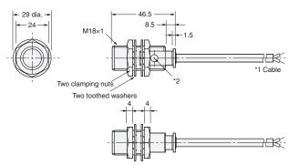
\*1 6-dia. vinyl-insulated round cable with 2 conductors (Conductor cross section: 0.5 mm², Insulator diameter: 1.9 mm), Standard length: 2 m.
